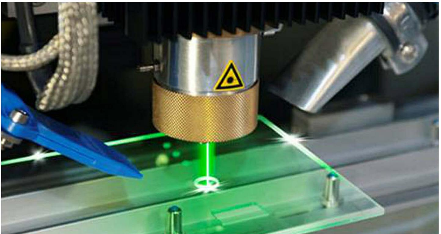
The light produced in a resonator is directed to the surface of a sample via an optical transmission system (mirror systems or fiber optics).
